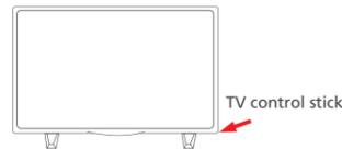
Switch on the television by pressing the TV control stick located on the TV set.
