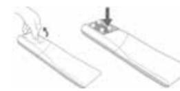
Insert the batteries supplied into the remote control and press the standby button to power on the TV.
