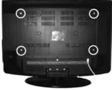
1) Remove the four screws highlighted below.
