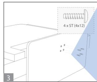
3 Secure the base to the neck by using the 4 x ST(4x12) screws provided.
