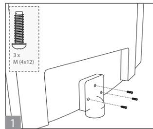
1 Attach the stand neck to the rear of the TV set using the 3 x M(4x12) screws.
