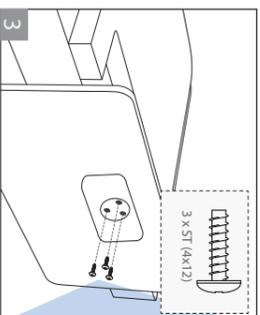
Secure the base to the neck by using the 4 x ST(4x12) screws provided.
