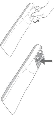
Remove the battery cover from the rear of the remote control and insert the AAA batteries which are supplied in the accessory pack. Ensure that the polarity of the batteries is as shown in the battery compartment. Replace the battery cover. The remote control is ready for use.
