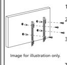
1) Remove the four screws that are supplied in the wall mounting holes. 2) The wall mount can now be easily attached to the mounting holes on the rear of the TV.
